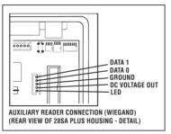
This cable may be extended up to 500' by splicing in additional wire. Note that the Data 1 uses the White wire at position #1.
