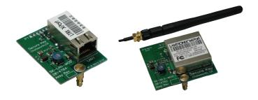
Secura Key's Network Modules allow the SK-ACP to easily connect to your Local Area Network, so that you can use your existing network infrastructure to monitor and control your access control system. You have your choice of SK-LAN-MOD for 10/100 Base-T Ethernet connections or the SK-WLS MOD for 802.11b/g wireless.
