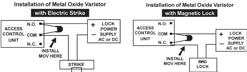
Figure 2 - MOV Wiring Diagram
