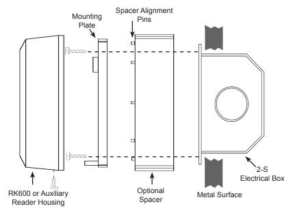
Figure 5 - Wall Mounting on Metal Surface with Optional Spacer
