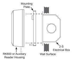
Figure 4 - Basic Installation
