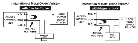
Figure 2 - MOV Wiring Diagram
