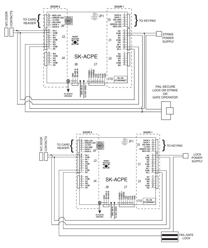
NOTES: Where dual-credential is required during just certain hours or days of the week, you may use the auxiliary output, defined as a "Time Zone" activated, to shunt either the keypad or the card reader during single-credential time periods.
