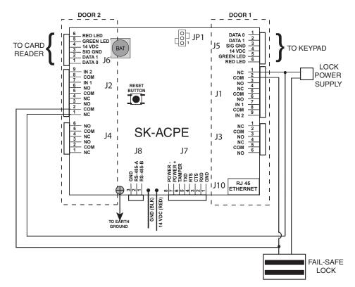
NOTES: Each valid access will appear as two valid access messages in SK-NET. Set the latch timers long enough to allow the user to present his card after entering his PIN and still have time to get the door open.
