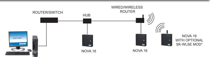
ETHERNET CABLE: (Required cables CAT 5e or CAT 6). Wired: max distance 300' (100m) between devices. Wireless: Typically 100-200' (30-60m) depending on interference, building structure and metal objects.
