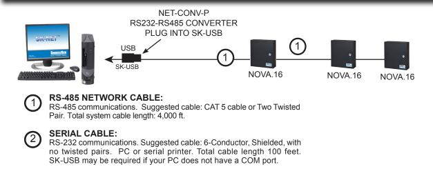
**Note:** When using the RS-232 to RS-485 converter, you cannot use the stubbed, star fanout or "T" configuration. All network connections from SK-MRCP to the next SK-MRCP must be in parallel with each other. The J2 connector, Pins 1 and 2 must be a twisted pair. Pin 3 (Ground) uses a conductor from another pair, if you are using CAT 5 or CAT 6 cable .
